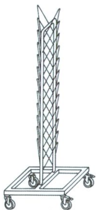
EMAX-8100 moving holder for 20 covers high: 1800
